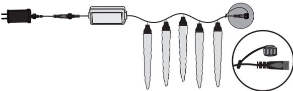
6. Connect the two kits together. Tighten the lock nut to secure the connection.
