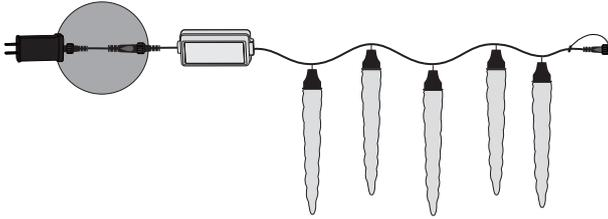
2. Unlock the lock nut, and pull apart the plugs to reveal the male connector.
