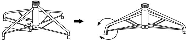
To close the stand, press the metal button and fold the legs together.
