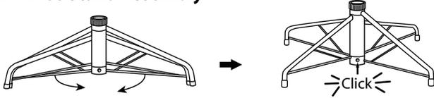
Pull apart the legs of the stand so that they are snapped into an x-shape, place the tree stand on a level surface.
