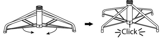
**Step 3.** To close the stand, press the metal button and fold the legs together.
