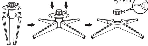
1. Unfold the legs and lay the stand in a flat area. Then slide the locking disc downward and snap into place.
