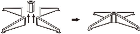
Insert and slide the legs upward into the slots of the base until firmly secured.
