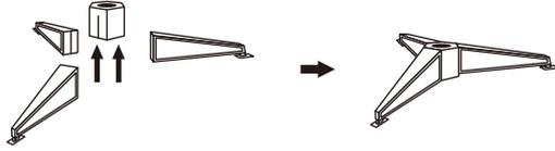
Insert and slide the legs upward into the slots of the base until firmly secured.
