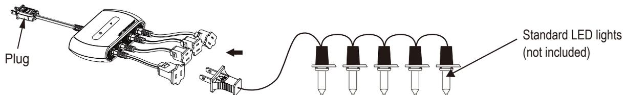
2. Plug the product to a wall or electrical outlet. If an extension cord is needed, you may connect it either at position ❶ (between the electrical outlet and product's main plug) or position ❷ (between one of the four outlets and light string's plug).
