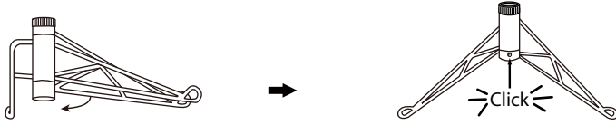
Fig. A - Tree Stand Assembly
