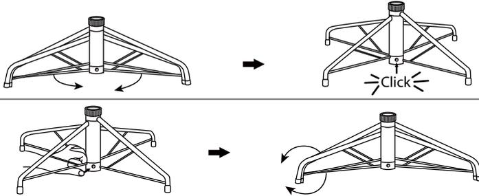
Pull apart the legs of the stand so that they are snapped into an x-shape, place the tree stand on a level surface.
