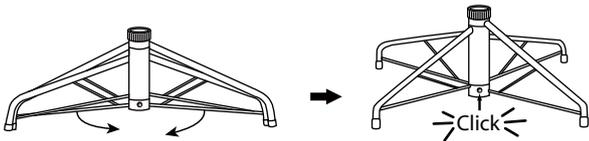
Pull apart the legs of the stand so that they are snapped into an x-shape. Place the tree stand on a level surface.
