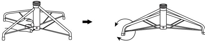
To close the stand, press the metal button and fold the legs together.
