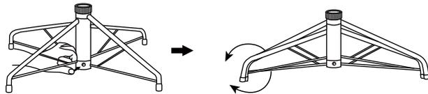
To close the stand, press the metal button and fold the legs together.
