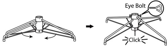
To close the stand, remove the eyebolts, press the metal button and fold the legs together.
