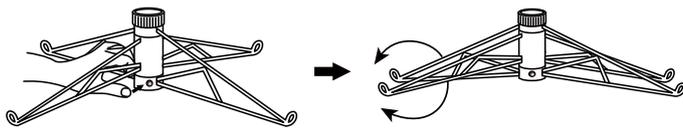
To close the stand, press the metal button and fold the legs together.
