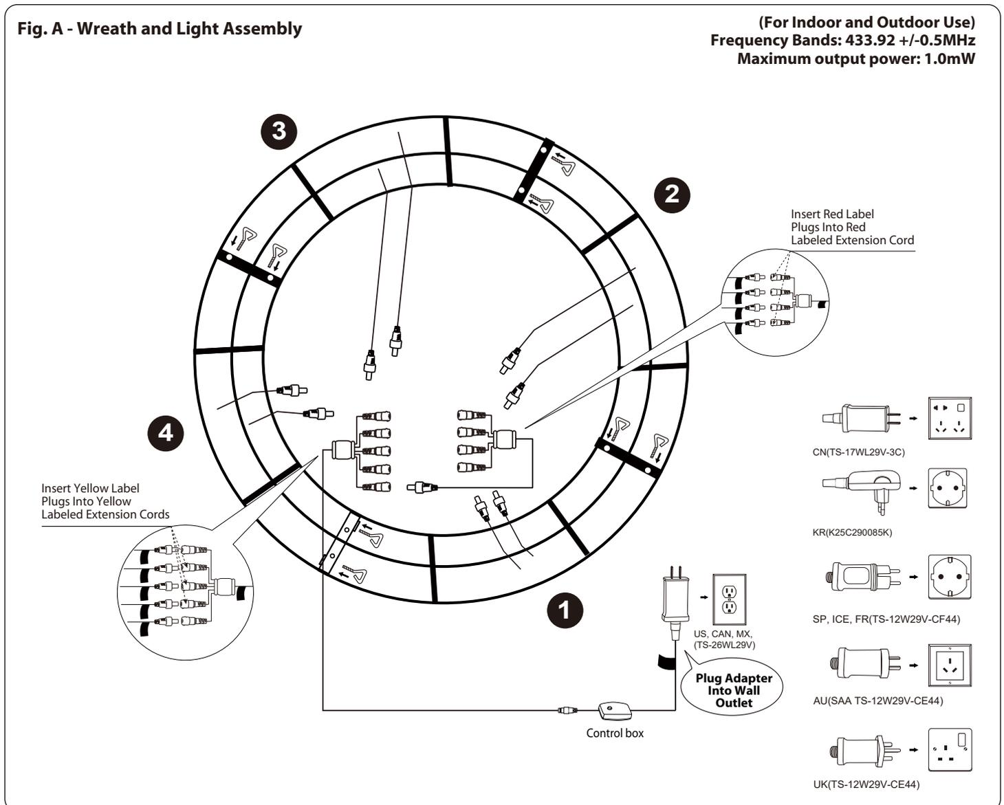
3. Assemble the wreath as shown in **Fig. A**.
