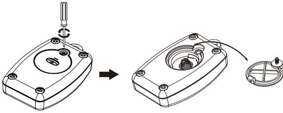
2. Replace the used battery with a new CR2032 button cell battery (not included). Make sure that the battery is installed with the correct polarity (+ and -).
