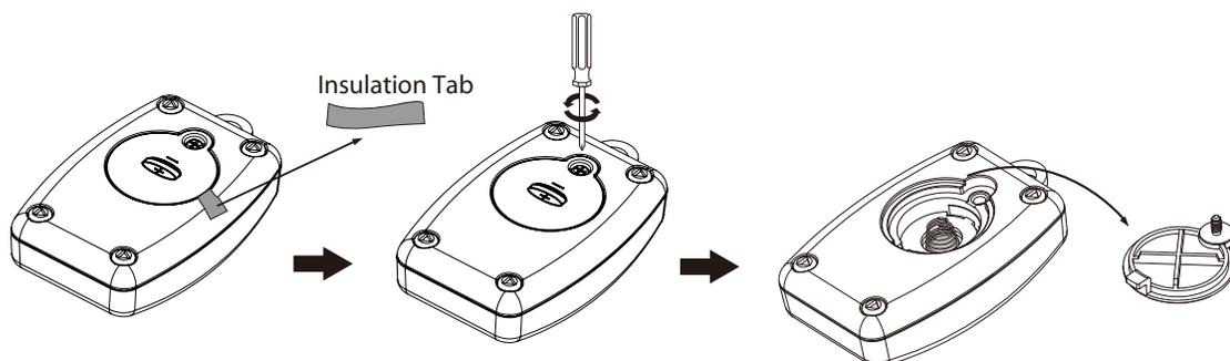
3. Replace the used battery with a new CR2032 button cell battery (not included). Make sure that the battery is installed with the correct polarity (+ and -).
