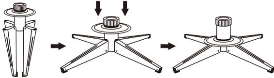
Unfold the legs and lay the stand in a flat area. Then slide the locking disc downward and snap into place.
