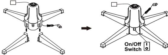
Slide the legs upwards into slots at the base of the trunk and tap lightly with hammer until firmly fixed.
