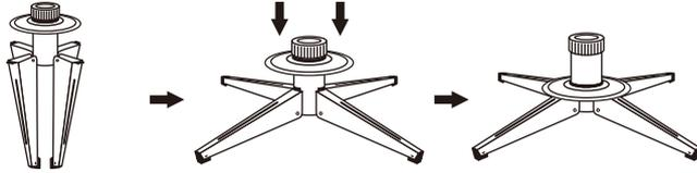
Unfold the legs and lay the stand in a flat area. Then slide the locking disc downward and snap into place.
