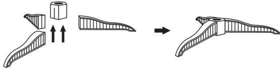
Insert and slide the legs upward into the slots of the base until firmly secured.
