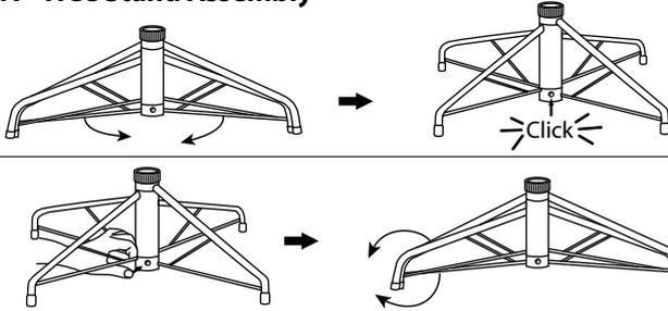
Pull apart the legs of the stand so that they are snapped into an x-shape, place the tree stand on a level surface.
