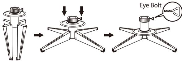
1. Unfold the legs and lay the stand in a flat area. Then slide the locking disc downward and snap into place.
