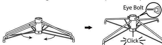
To close the stand, remove the eyebolts, press the metal button and fold the legs together.
