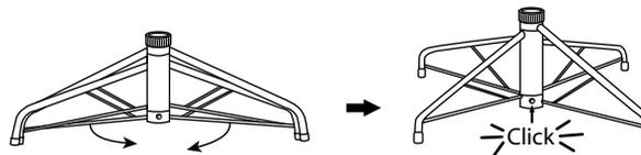
To close the stand, remove the eyebolts, press the metal button and fold the legs together.
