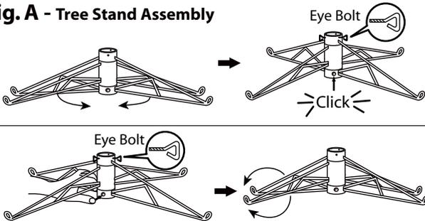
1. Pull apart the legs of the stand so that they are snapped into an x-shape, place the tree stand on a level surface.
