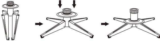
Unfold the legs and lay the stand in a flat area. Then slide the locking disc downward and snap into place.
