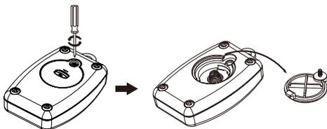
2. Replace the used battery with a new CR2032 button cell battery (not included). Make sure that the battery is installed with the correct polarity (+ and -).
