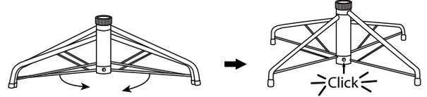
**Step 3.** To close the stand, press the metal button and fold the legs together.
