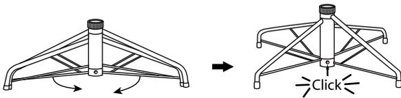
Swivel the legs of the stand until they snap into position. (The legs should be evenly spaced once this step is complete). place the tree stand on a level surface.
