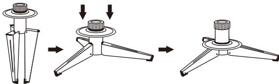
Unfold the legs and lay the stand in a flat area. Then slide the locking disc downward and snap into place.
