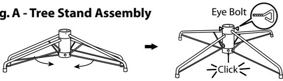
1. Pull apart the legs of the stand so that they are snapped into an x-shape, place the tree stand on a level surface.
