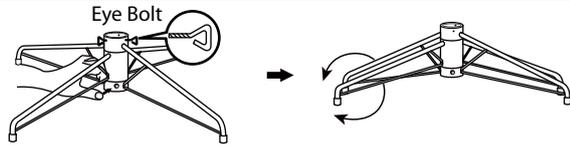
To close the stand, remove the eyebolts, press the metal button and fold the legs together.
