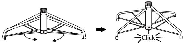
Pull apart the legs of the stand so that they are snapped into an X-shape, and place the tree stand on a level surface.
