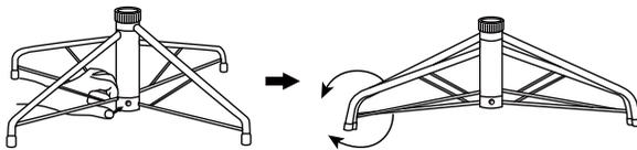
To close the stand, press the metal button and fold the legs together.
