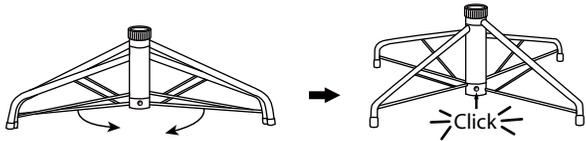
Pull apart the legs of the stand so that they are snapped into an X-shape, and place the tree stand on a level surface.
