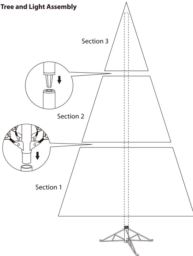
3. Each tree section is numbered with a tag. Please identify all sections before assembling.
